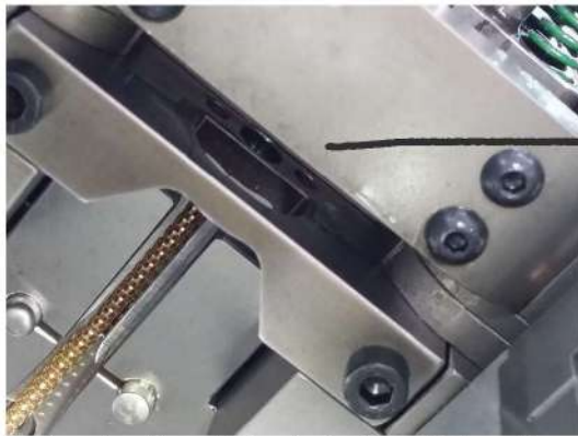
Tooling die with cartridge design for quick inserting
